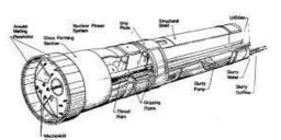
nuclear reactor that circulates liquid lithium from the reactor core to the tunnel face, where it melts the rock.
